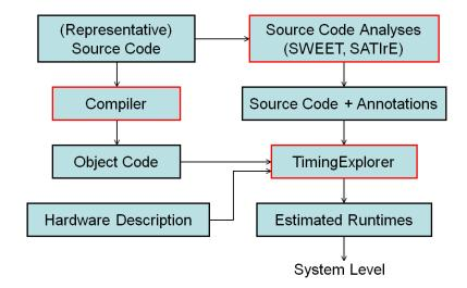
Figure 11: Workflow for source-code analysis and static timing analysis.
